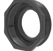
Converts 1.5" Standard Union Thread to Larger Hayward FINE Union Thread
